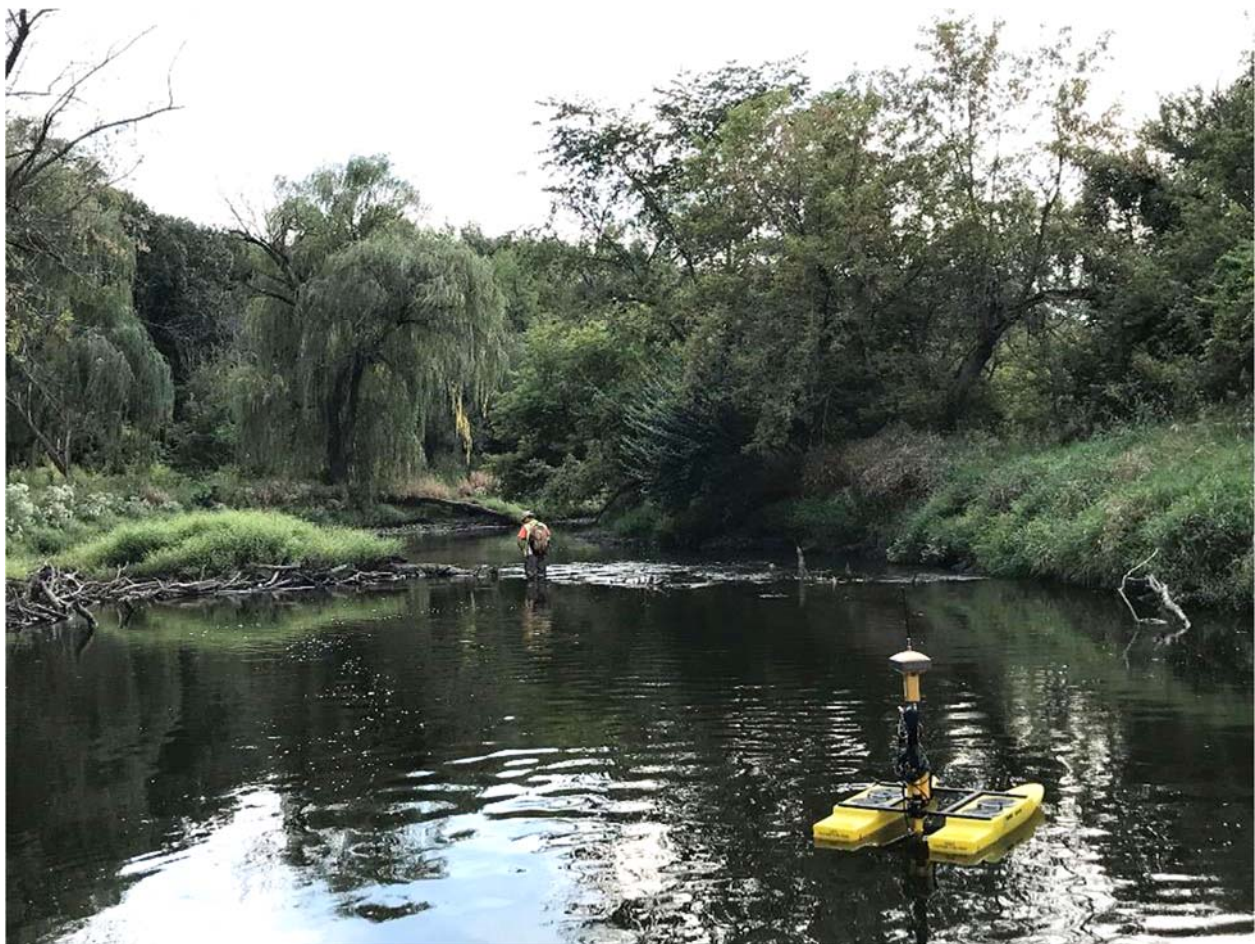
Figure 6. Image of the HyDrone equipped with single-beam sonar and RTK-GPS equipment in operation upstream of Trout Farm Park
